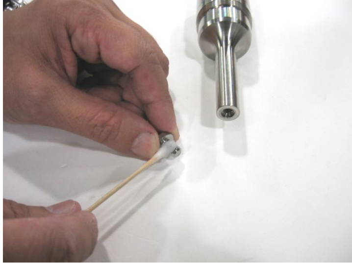
Cleaning replaceable tip threading
